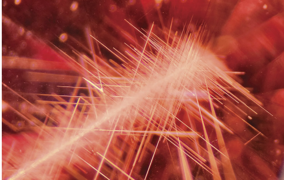
Figure 4. A collection of needle inclusions in a 2.30 ct pyrope-almandine garnet. Photomicrograph by Isabelle Corvin; field of view 2.5 mm.
